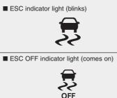
When the ignition switch is pressed to the ON position, the ESC indicator light illuminates, then goes off if the ESC system is operating normally.
