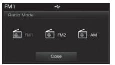
Turn the  $\bigcirc$  TUNE knob to move the focus. Press the knob to select.
