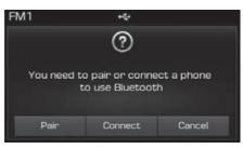
If *Bluetooth*<sup>®</sup> Wireless Technology devices are paired but none are currently connected, pressing the PHONE key or the key on the steering remote controller displays the following screen. Press the [Pair] button to pair a new device or press the [Connect] to connect a previously pair device.
