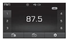
Press the field button to display the broadcast information for the frequency saved to each button.
