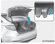
The trunk lid control switch is used to prevent unauthorized access to the trunk.
