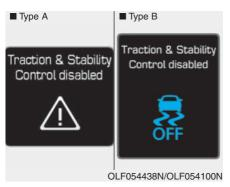
Press the ESC OFF button for more than 3 seconds. ESC OFF indicator light and message illuminates and ESC OFF warning chime will sound. At this state, the engine control function and brake control function does not operate. In other words, the vehicle stability control function does not operate any more.
