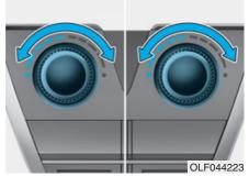
Turn the temperature control knob to set the desired temperature.
