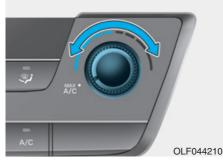
The temperature control knob allows you to control the temperature of the air flowing from the ventilation system. To change the air temperature in the passenger compartment, turn the knob to the right position for warm and hot air or left position for cooler air.
