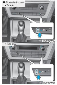
The seat warmers and air ventilation seats are provided to warm or cool the front seats by blowing air through small vent holes on the surface of the seat cushions and seatbacks.
