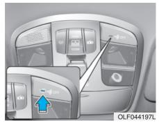
The intrusion/tilt sensor detects movement inside the vehicle and inclination of the vehicle after locking.
