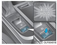
1. With the driver's door, engine hood and trunk closed, fasten the driver's seat belt or depress the brake pedal and then press the [AUTO HOLD] switch. The white AUTO HOLD indicator will come on and the system will be in the standby position.
