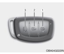
Your HYUNDAI uses a Smart Key, which you can use to lock or unlock a door (and trunk) and even start the engine.
