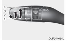
To operate the lights, turn the knob at the end of the control lever to one of the following positions:
