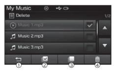
Press the button or individually select the files you want to delete. Once files are selected, the button and minimum buttons will be enabled.
