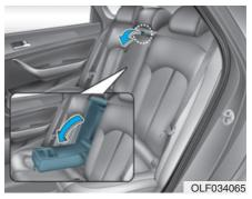
The armrest is located in the center of the rear seat. Pull the armrest down from the seatback to use it.
