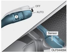
The rain sensor located on the upper end of the windshield glass senses the amount of rainfall and controls the wiping cycle for the proper interval. The more it rains, the faster the wiper operates.
