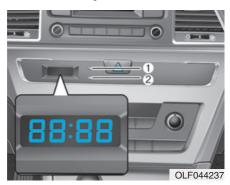
Whenever the battery terminals or related fuses are disconnected, you must reset the time.
