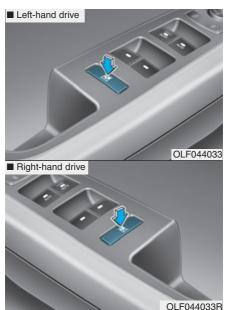
The driver can disable the power window switches on the rear passengers' doors by pressing the power window lock switch When the power window lock switch is pressed:
