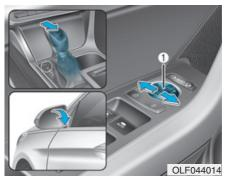
When you move the shift lever to the R (Reverse) position, the outside rearview mirror(s) will rotate downwards to aid with driving in reverse.
