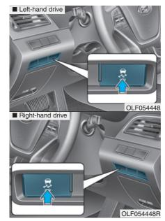
The Electronic Stability Control (ESC) system helps to stabilize the vehicle during cornering maneuvers.
