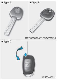
If the remote key does not operate normally, you can lock or unlock the door by using the mechanical key.
