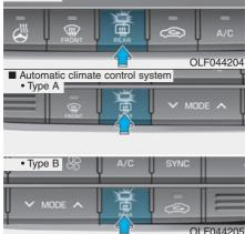
The defroster heats the window to remove frost, fog and thin ice from the interior and exterior of the rear window, while engine is running.
