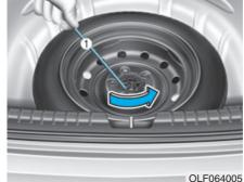
If it is hard to loosen the tire holddown wing bolt by hand, you can loosen it easily using the jack handle.
