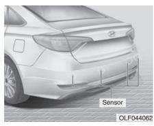
The Rear Parking Assist System aids the driver during backward movement of the vehicle by chiming if any object is sensed within the distance of about 120 cm (47 in.) behind the vehicle. This is a supplemental system that senses objects within the range and location of the sensors, it cannot detect objects in other areas where sensors are not installed.
