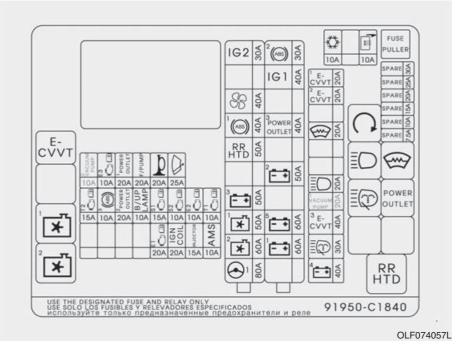
Engine compartment main fuse panel
