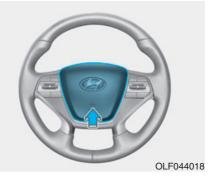
To sound the horn, press the area indicated by the horn symbol on your steering wheel (see illustration). The horn will operate only when this area is pressed.
