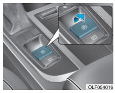
To apply the EPB (Electric Parking Brake):
