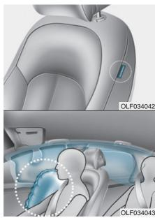
Your vehicle is equipped with a side air bag in each front seat. The purpose of the air bag is to provide the vehicle's driver and the front passenger with additional protection than that offered by the seat belt alone. The side air bags are designed to deploy only during certain side impact collisions, depending on the crash severity, angle, speed and point of impact.
