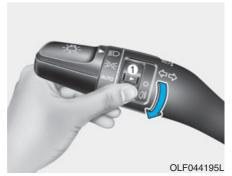
Vehicle without front fog lamp To turn on the rear fog lamp:
