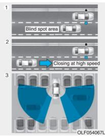
The Blind Spot Detection System (BSD) uses a radar sensor to alert the driver.
