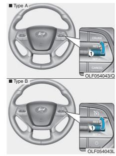
• Push the lever (1) up (RES+) and hold it, while monitoring the SET speed on the instrument cluster.
