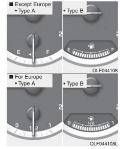
This gauge indicates the approximate amount of fuel remaining in the fuel tank.
