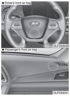
The purpose of the SRS is to provide the vehicle's driver and front passengers with additional protection than that offered by the seat belt system alone in case of a frontal impact of sufficient severity.
