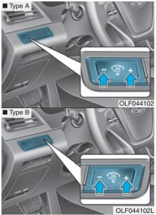
When the vehicle's parking lights or headlights are on, press the illumination control button to adjust the brightness of the instrument panel illumination. When pressing the illumination control button, the interior switch illumination intensity is also adjusted. The selected brightness of illumination can be saved in the Driver position memory system(if equipped).
