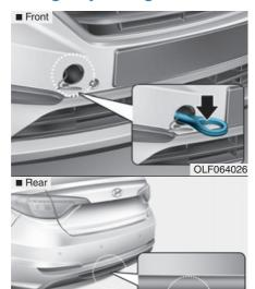
If towing service is not available in an emergency, your vehicle may be temporarily towed using a cable or chain secured to the emergency towing hook at the front (or rear) of the vehicle.
