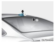
*Shark fin antenna (1, if equipped)* The shark fin antenna will receive the transmit data.
