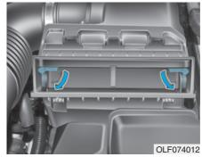
3. Pull down the lever to the UNLOCK position.
