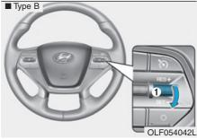
Push the lever (1) up (RES+). If the vehicle speed is over 40 km/h (25 mph), the vehicle will resume the preset speed.
