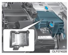
Inside the fuse/relay box covers, you can find the fuse/relay label describing fuse/relay name and capacity.
