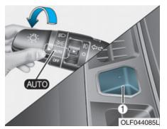
AUTO light position (if equipped) When the light switch is in the AUTO position, the parking lamp and headlamp will be turned ON or OFF automatically depending on the amount of light outside the vehicle.
