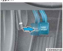
Check whether the stroke is within specification when the parking brake pedal is depressed with 20 kg (44 lb, 196N) of force. Also, the parking brake alone should securely hold the vehicle on a fairly steep grade. If the stroke is more or less than specified, we recommend that the system be serviced by an authorized HYUNDAI dealer.
