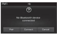
• If *Bluetooth*<sup>®</sup> Wireless Technology devices are paired but none are currently connected, pressing the key or the key on the steering remote controller displays the following screen. Press the [Pair] button to pair a new device or press the [Connect] to connect a previously pair device.
