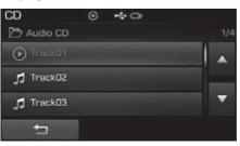
Turn the **OTUNE** knob left/right to search for tracks. Once the desired track is displayed, press the knob to select and play.
