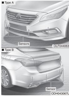
The Parking Assist System assists the driver during movement of the vehicle by chiming if any object is sensed within the distance of 100 cm (39 inches) in front and 120 cm (47 inches) behind the vehicle. This system is a supplemental system that senses objects within the range and location of the sensors, it cannot detect objects in other areas where sensors are not installed.
