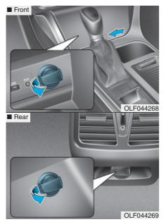
The power outlet is designed to provide power for mobile telephones or other devices designed to operate with vehicle electrical systems. The devices should draw less than 180 W(Watt) with the engine running.
