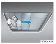
If an object or part of the body is detected while the sunroof glass or sunshade is closing automatically, it will reverse the direction, and then stop.
