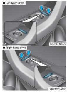
Electric type (if equipped) Left : The mirror will unfold. Right : The mirror will fold.
