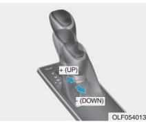
Whether the vehicle is stationary or in motion, sports mode is selected by pushing the shift lever from the D (Drive) position into the manual gate. To return to D (Drive) range operation, push the shift lever back into the main gate. In Sports Mode, moving the shift lever backwards and forwards will allow you to select the desired range of gears for the current driving conditions.
