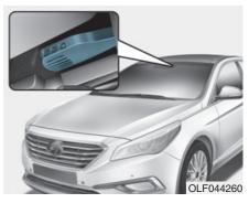
Auto defogging reduces the possibility of fogging up the inside of the windshield by automatically sensing the moisture of inside the windshield.
