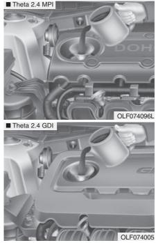
If it is near or at L, add enough oil to bring the level to F. **Do not overfill.** Use a funnel to help prevent oil from being spilled on engine components.
