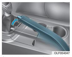
Check the stroke of the parking brake by counting the number of "clicks" heard while fully applying it from the released position. Also, the parking brake alone should securely hold the vehicle on a fairly steep grade. If the stroke is more or less than specified, we recommend that the system be serviced by an authorized HYUNDAI dealer.
