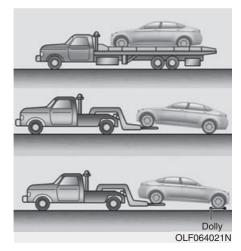
If emergency towing is necessary, we recommend having it done by an authorized HYUNDAI dealer or a commercial tow-truck service. Proper lifting and towing procedures are necessary to prevent damage to the vehicle. The use of wheel dollies or flatbed is recommended. It is acceptable to tow the vehicle with the rear wheels on the ground (without dollies) and the front wheels off the ground.
