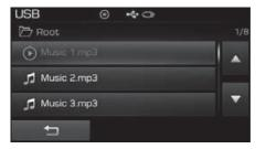
Turn the **O**TUNE knob left/right to search for files. Once the desired file is displayed, press the knob to select and play.
