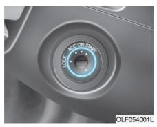
Whenever the front door is opened, the ignition switch will illuminate, provided the ignition switch is not in the ON position. The light will go off immediately when the ignition switch is turned on or go off after about 30 seconds when the door is closed. (if equipped)
