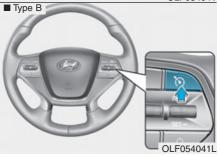
1. Push the CRUISE / 🏷 button on the steering wheel to turn the system on. The CRUISE indicator will illuminate.
