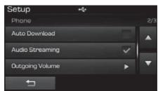
This feature is used to automatically download mobile contacts entries once a *Bluetooth*<sup>®</sup> Wireless Technology phone is connected.
