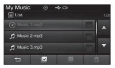
Turn the **O**TUNE knob left/right to search for files. Once the desired file is displayed, press the knob to select and play.
