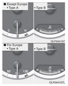
This gauge indicates the temperature of the engine coolant when the ignition switch or Engine Start/Stop button is in the ON position.
