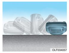
Front air bags may not inflate in rollover accidents because front air bag deployment would not provide additional occupant protection.
