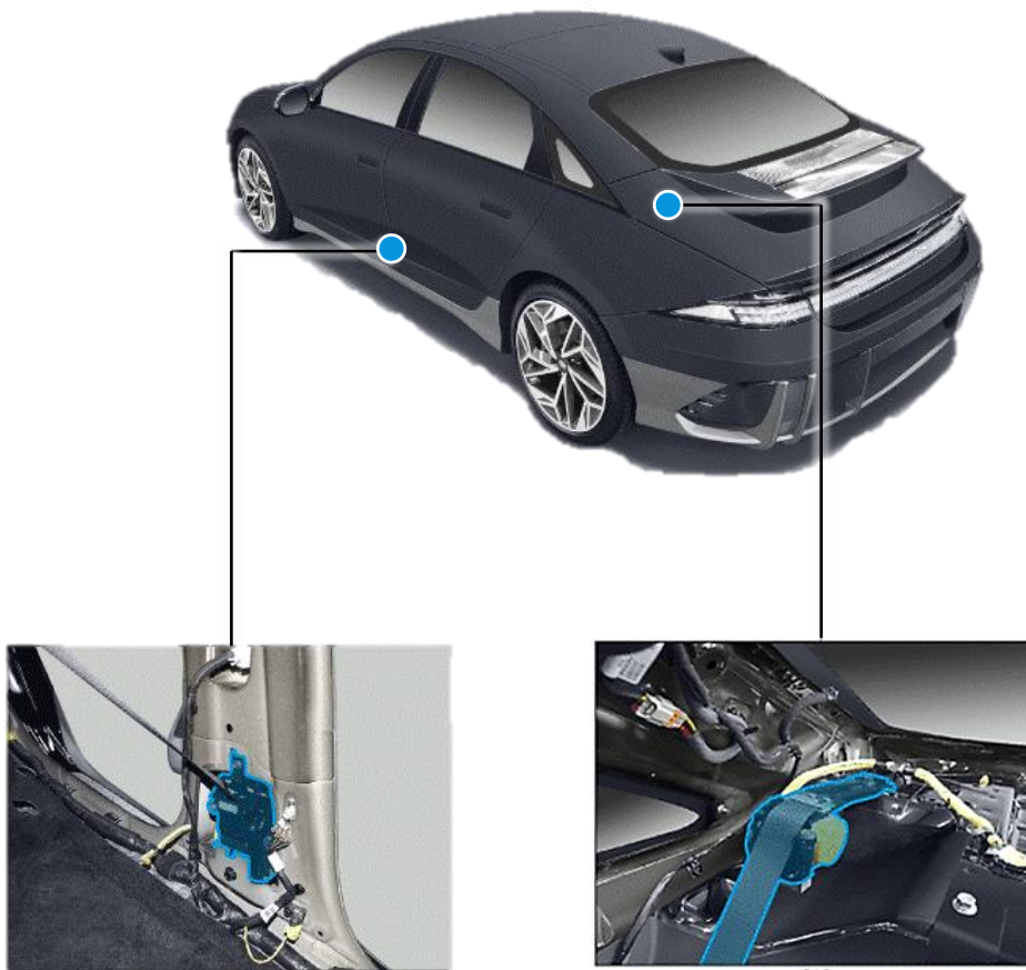
1) Front Seatbelt Pretensioner
