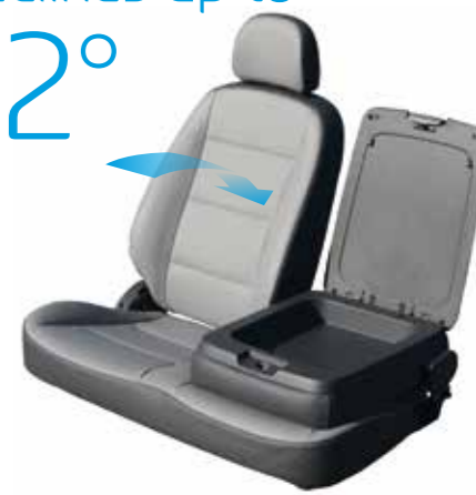
Reclining Passenger Seat and Folding Console The Super Cab passenger seat reclines up to a maximum of 52 degrees (degrees in Standard Cab). For added convenience, the center seat backrest can be folded into a fully flat position to offer a handy 6 liter storage compartment. It's covered by a large tray top doubles as a writing surface.
