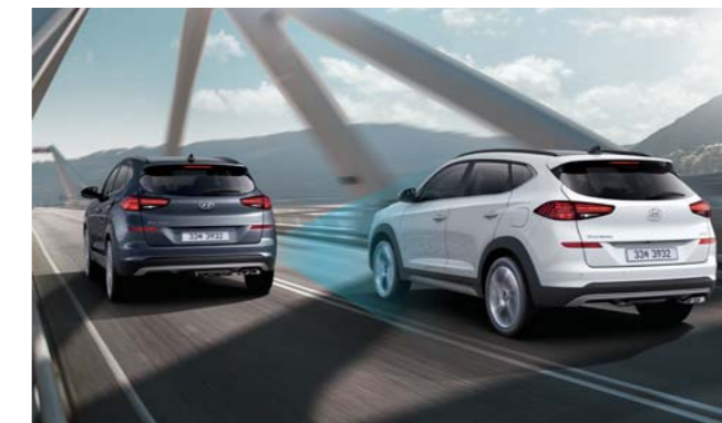
High Beam Assist This feature reduces the inconvenience of frequently using the high beam controls by automatically switching high beams to low beams when there are cars in front or driving in the opposite lane. Blind-spot Collision Warning Reduces risk of collision by detecting and warning the driver of vehicles approaching from the rear or in the vehicle's blind spot that cannot be seen through the side mirrors.
