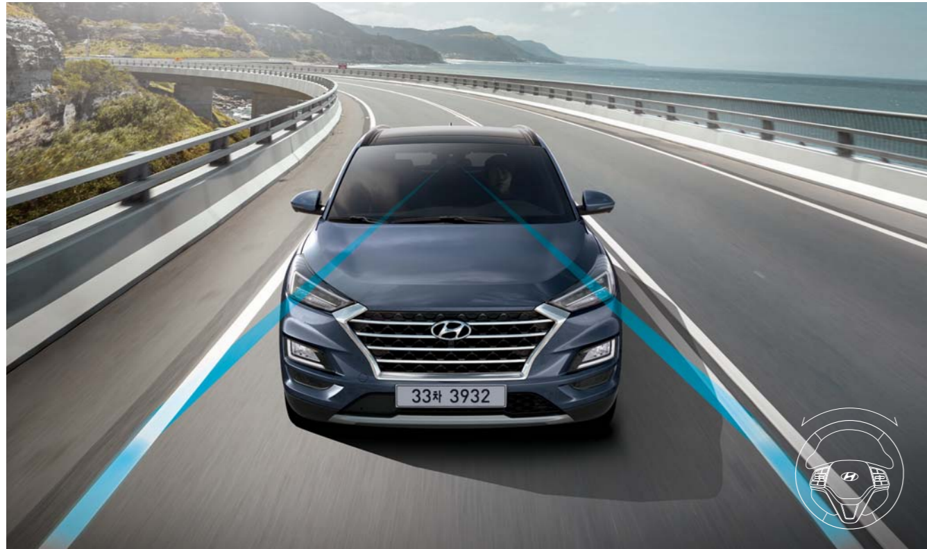
Lane Keeping Assist / Lane Departure Warning Recognizes the boundaries of the current lane using the front camera and gives a warning or adjusts the steering if the vehicle seems to be about to depart the lane without prior turn signal activation.
