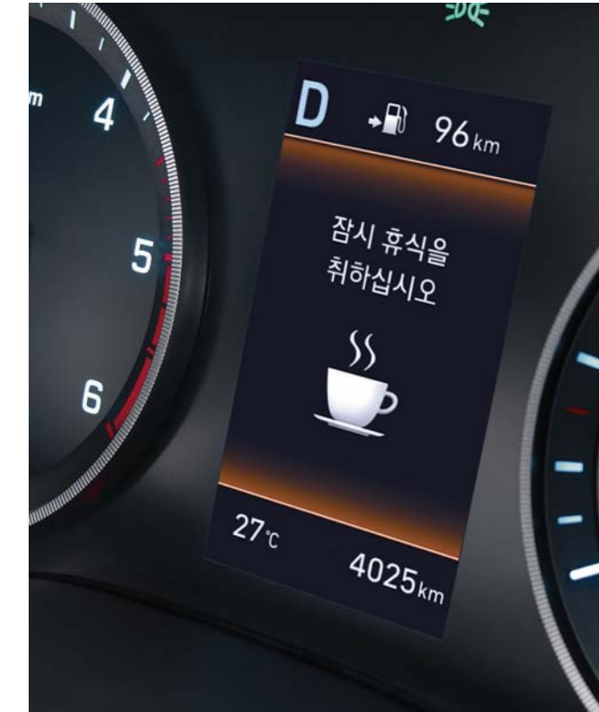
Driver Attention Warning The vehicle comprehensively analyzes the driver's driving patterns and its position in a lane and, when driver fatigue or negligent driving detected, a popup message is issued together with an alert sound to recommend the driver to take a break.
