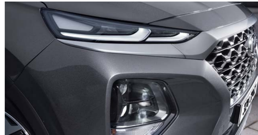
Cascading grille LED Daytime Running Light (DRL, with positioning function), Bi-function LED headlamp
