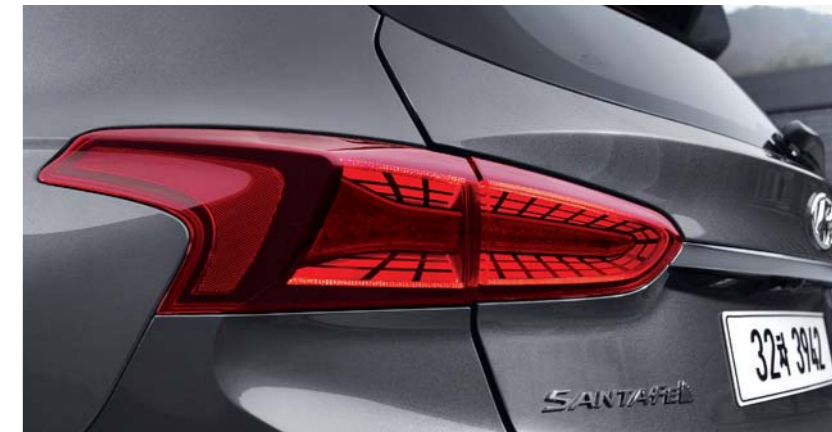
Door chrome garnish LED tail light (with brake light and tail light)
