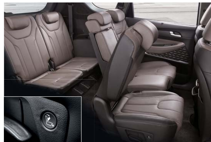
Second row smart one touch walk-in Upon pressing the walk-in button located at the base of the second row seat, the back of the seat will fold forward. The seat itself will also move forward, giving those sitting in the third row ample room to get in and out of the vehicle.
