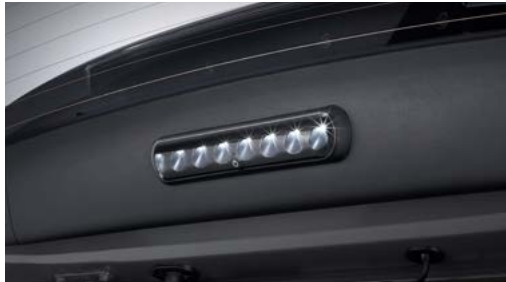
LED tailgate lamp(touch-activated)
