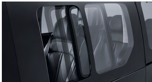
Acoustic Laminated Glass for the front row Flush Glass
