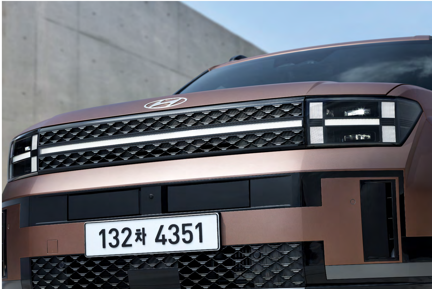
Horizontal LED Lamp (Positioning Lamp) & Full LED Headlamps (Projection Type)
