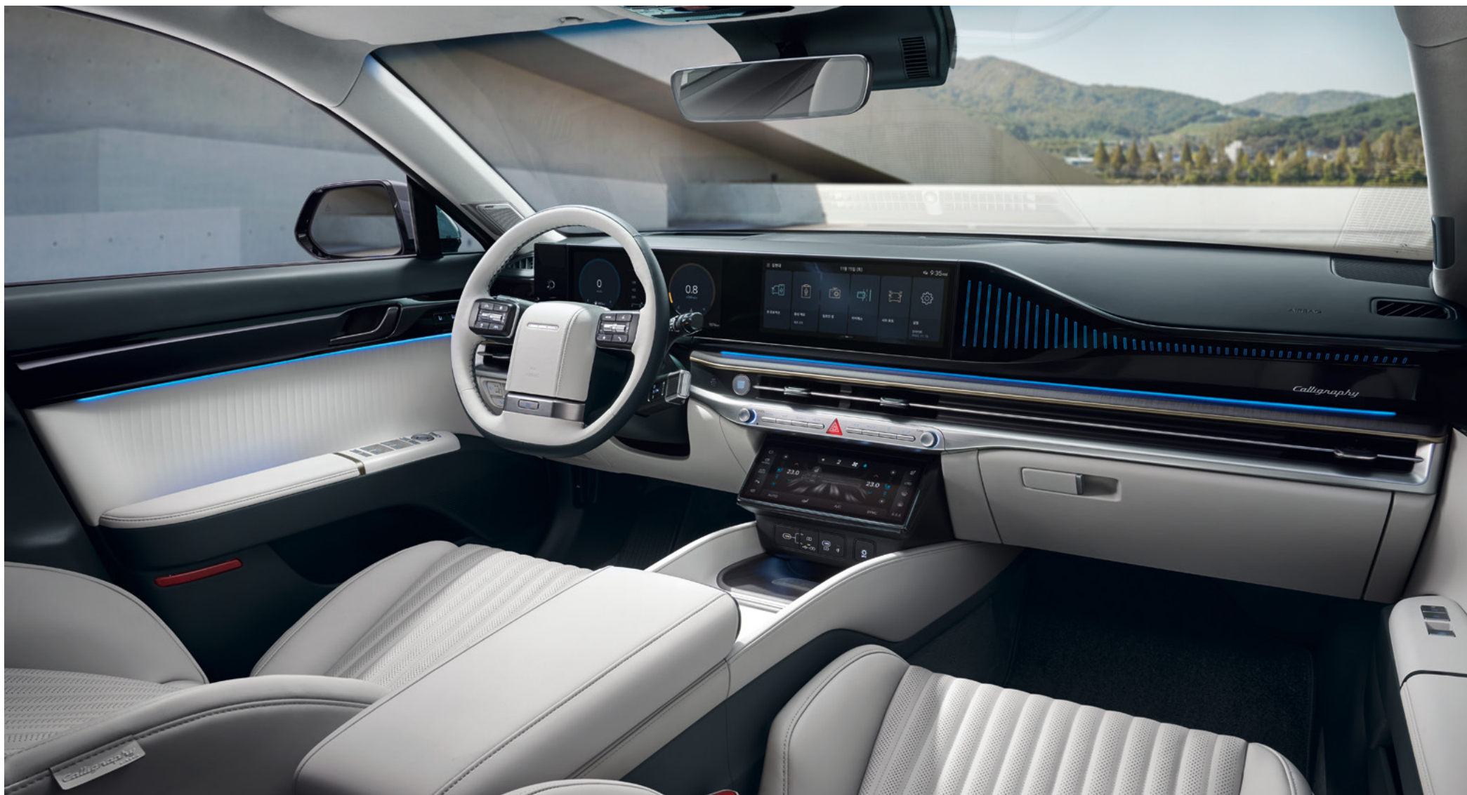
Calligraphy Full Option (Indigo/Light Gray two-tone): Bezel-less inside mirrors, antibacterial-treated interior materials, suede interior materials, interactive ambient mood lamp, power tilt & telescopic steering wheel (including vibration warning, heating, and interactive light), electronic shift column, Hyundai Motor's next-generation infotainment system (ccNC), door trim-wide full armrest, 10.25" full-touch air conditioning controller (including Haptic controls)
