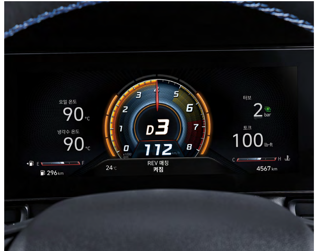
REV Matching During downshifts while driving, REV Matching synchronizes the engine and transmission revolutions to reduce shifting shocks, enabling quicker shifts and ensuring swifter reacceleration after deceleration.
