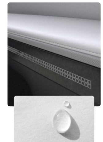
▶ 100% recyclable paperette detailing on the doors made from HDPE
