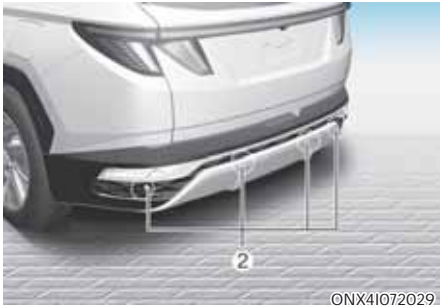
[2] : Rear ultrasonic sensors
