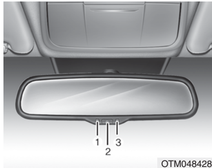
[1] : Indicator, [2] : ON/OFF button, [3] : Sensor
