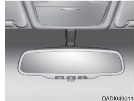
[1] : Indicator, [2] : ON/OFF button, [3] : Sensor
