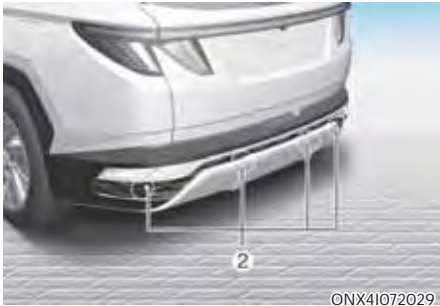
[2] : Rear ultrasonic sensors
