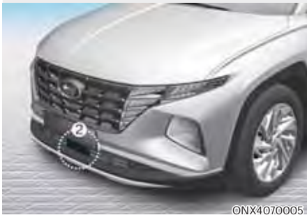
[1] : Front view camera, [2] : Front radar
