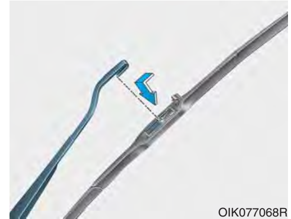
3. Install the new blade assembly in the reverse order of removal. 4. Return the wiper arm on the windshield.
