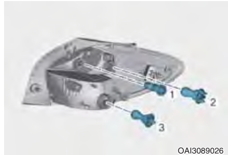
1 : Back Up Light 2 : Rear Turn Signal Light 3 : Tail and Stop Light
