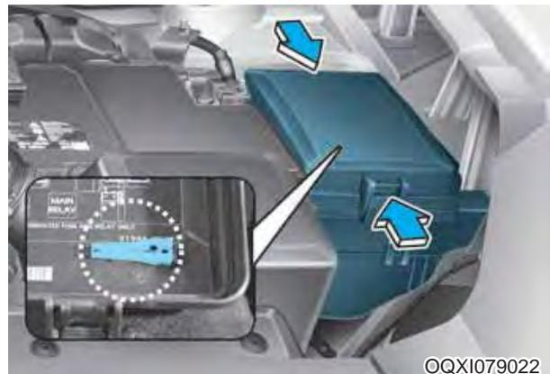
3. Pull the suspected fuse straight out. Use the fuse puller provided in the engine compartment fuse panel.
