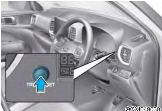
The trip computer is a microcomputer-controlled driver information system that displays information related to driving, when the ignition switch is in the ON position. All stored driving information (except odometer) resets if the battery is disconnected.
