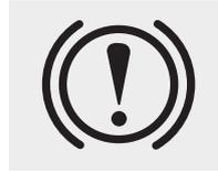
Check the Parking Brake Warning Light by placing the ignition switch to the ON position (do not start the engine).
