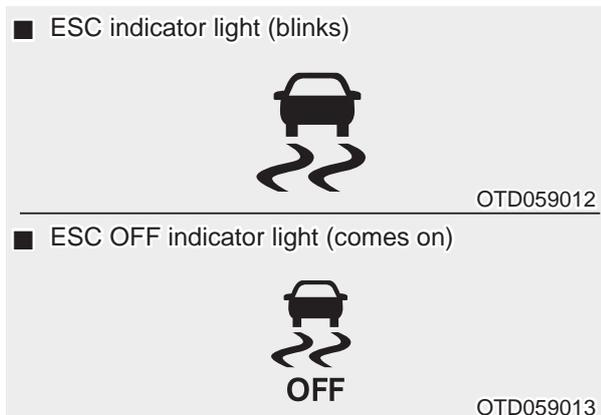
When the ignition switch is in the ON position, the ESC indicator light illuminates, then goes off if the ESC system is operating normally.
