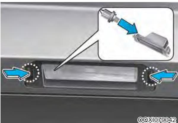
1. Using a flat-blade screwdriver, remove the light assembly from the body of the vehicle by prying the housing and pulling the assembly out.
