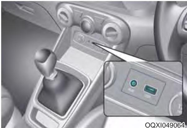
You can use an USB port to plug in an USB or an iPod®.
