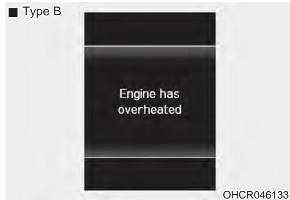
This warning message illuminates with a warning chime when the engine coolant temperature is above 120°C (248°F). This means that the engine is overheated and may be damaged.
