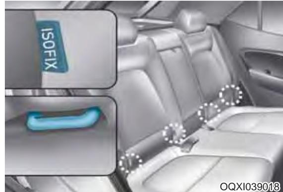
The ISOFIX anchorages symbols are located on the left and right rear seat cushions to identify the position of the ISOFIX anchorages in your vehicle (see arrows in illustration).
