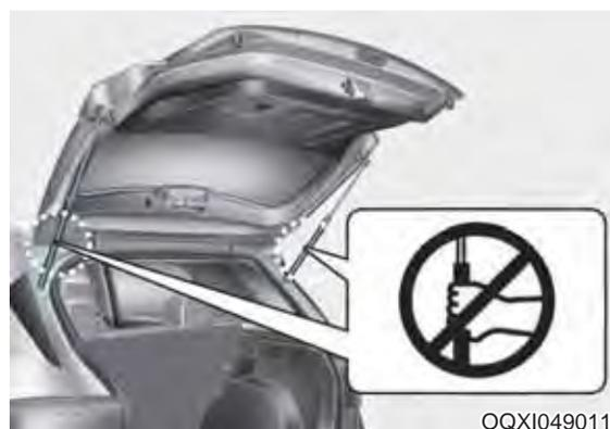
Do not hold the part (gas lifter) that supports the tailgate. Be aware that the deformation of the part may cause vehicle damage and a risk of safety accident.
