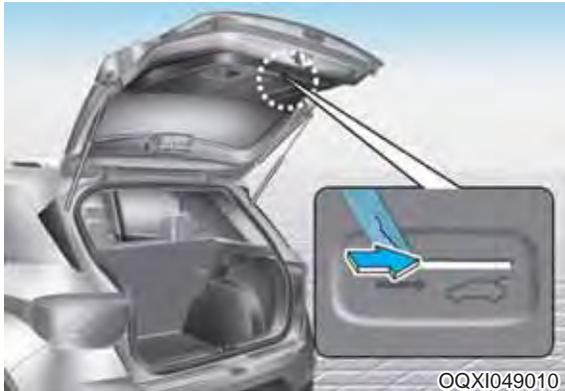
Your vehicle is equipped with the emergency tailgate safety release lever located on the bottom of the tailgate. When someone is inadvertently locked in the luggage compartment, the tailgate can be opened by doing as follows:
