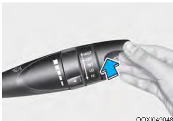
Push the lever away from you to spray rear washer fluid and to run the rear wipers 1~3 cycles. The spray and wiper operation will continue until you release the lever. (if equipped)
