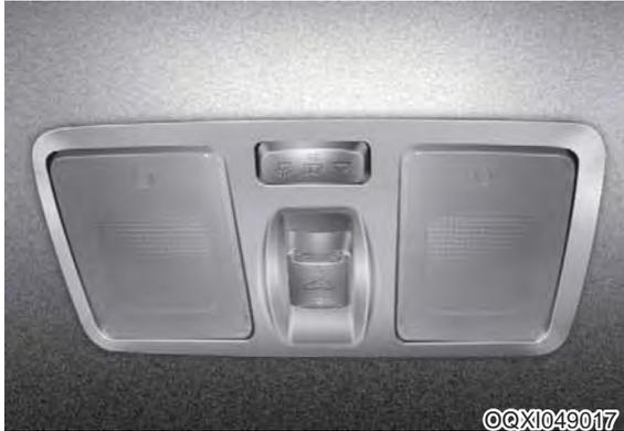
If your vehicle is equipped with a sunroof, you can slide or tilt your sunroof with the sunroof control switch located on the overhead console.
