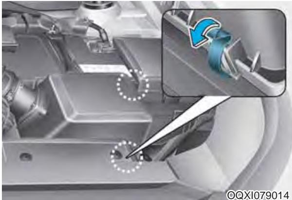
You can clean the filter when inspecting the air cleaner element.
