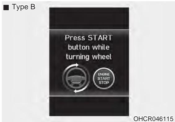
This warning message illuminates if the steering wheel does not unlock normally when the Engine Start/Stop button is pressed.
