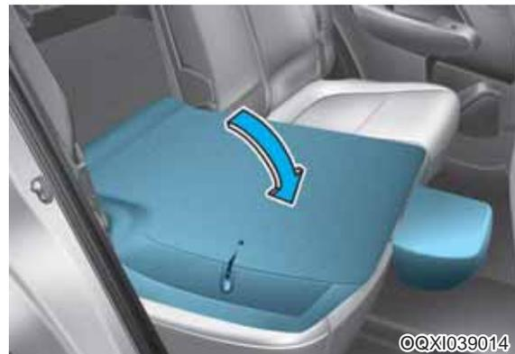
4. Pull up both sides of the seatback lever and fold the seatback toward the front of the vehicle.
