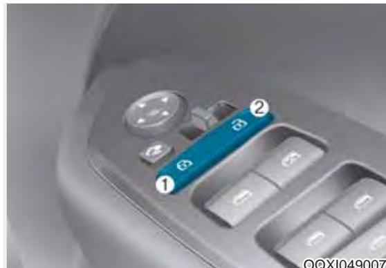
When pressing the (🔒) portion (1) of the switch, all vehicle doors will lock.
