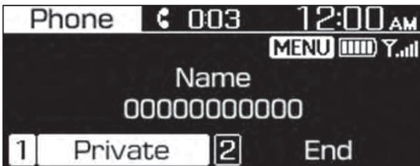
To switch the call to your mobile phone, press the [1 RPT] button on the control panel.
