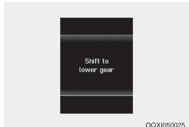
It is possible to drive on a slope with the gear is in first but the following warning message appears when the driver operates while the gear is in above second.
