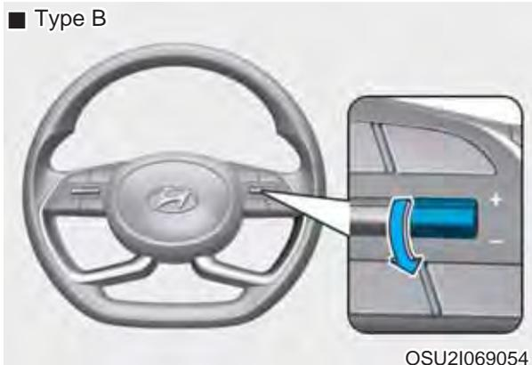
3. Push the toggle switch down (-), and release it. The SET indicator or set speed on the LCD display will illuminate.
