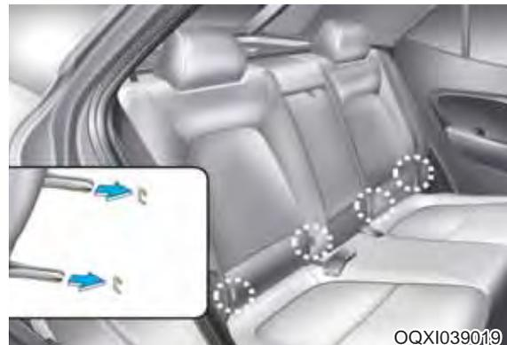
Both rear outboard seats are equipped with a pair of ISOFIX anchorages as well as a corresponding top-tether anchorage on the back side of the rear seats.
