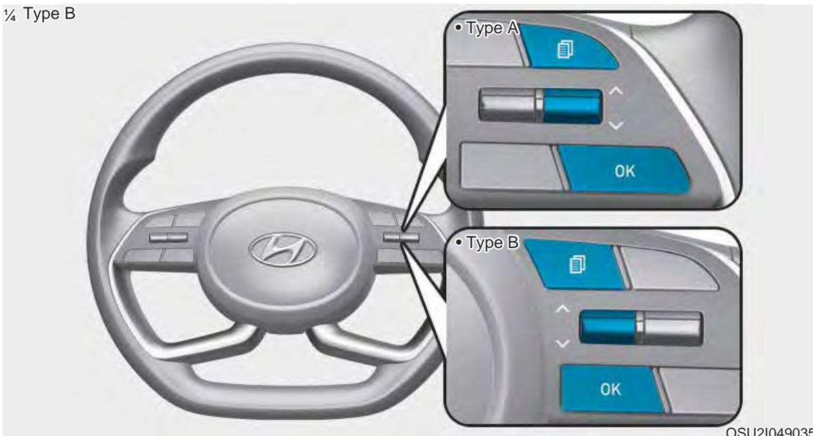
The LCD display modes can be changed by using the control buttons.
