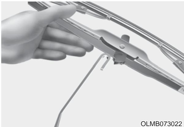
2. Compress the clip and slide the blade assembly downward.
