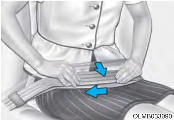
With a 2-point static type seat belt, the length must be adjusted manually so it fits snugly around your body. Fasten the belt and pull on the loose end to tighten. The belt should be placed as low as possible on your hips, not on your waist. If the belt is too high, it could increase the possibility of your being injured in an accident.
