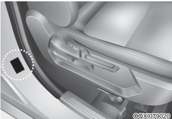
All specifications (sizes and pressures) can be found on a label attached to the vehicle.
