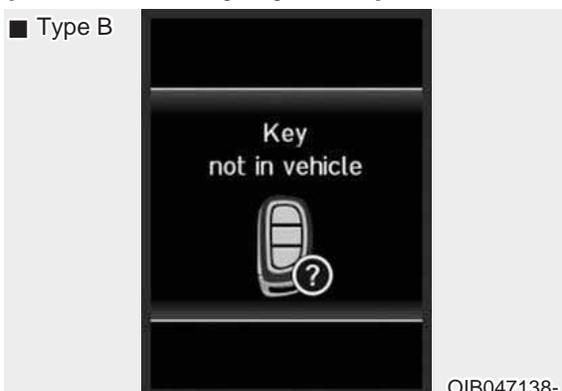
This warning message illuminates if the smart key is not in the vehicle when you press the Engine Start/Stop button.
