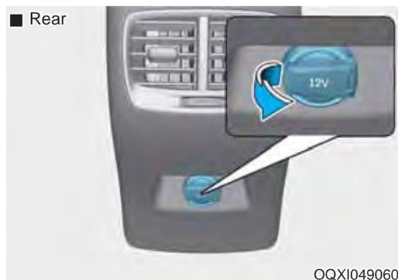
The power outlet is designed to provide power for mobile telephones or other devices designed to operate with vehicle electrical systems. The devices should draw less than 180W (Watt) with the engine running.
