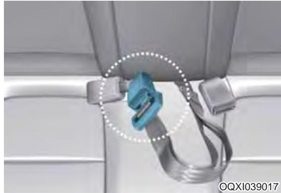
When using the rear center seat belt, the buckle with the “ENTER” mark must be used.
