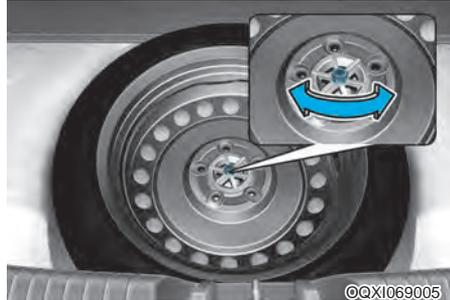
Turn the winged hold down bolt counterclockwise to remove the spare tire. Store the spare tire in the same compartment by turning the winged hold down bolt clockwise.
