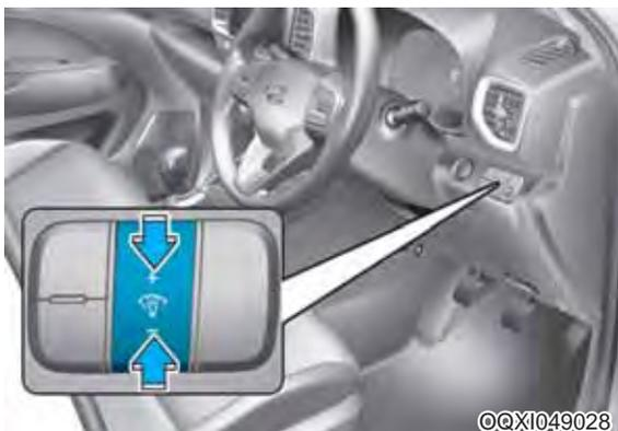
The brightness of the instrument panel illumination changes by pressing the upper or lower part of the switch when the ignition switch is in the ON position and when the parking lights are turned on.
