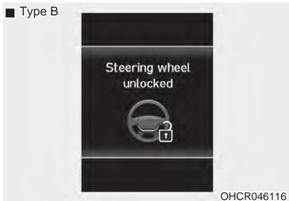
This warning message illuminates if the steering wheel does not lock when the Engine Start/Stop button is in the OFF position.
