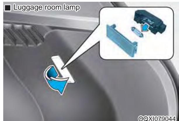
1. Using a flat-blade screwdriver, gently pry the lens from the interior light housing.
