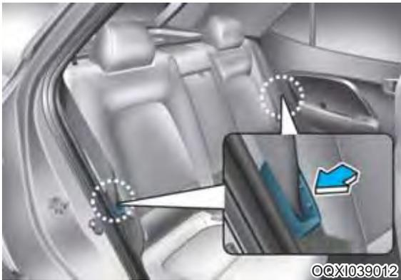
3. Insert the rear lap/shoulder belt plate into the holder on the side trim. It will prevent the lap/shoulder belt from interfering with the seatback when folding.
