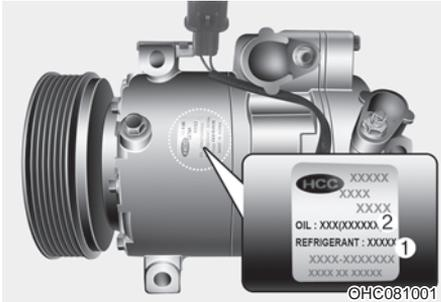
A compressor label informs you the type of compressor your vehicle is equipped with such as model, supplier part number, production number, refrigerant (1) and refrigerant oil (2).
