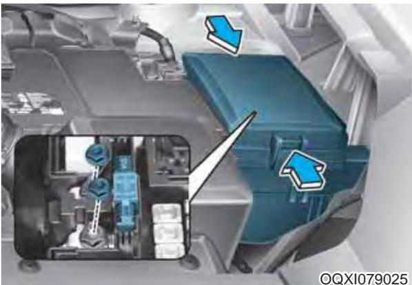
If the main fuse is blown, it must be removed as follows:
