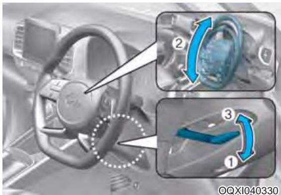
Pull down the lock-release lever (1) on the steering wheel column and adjust the steering wheel angle (2). Move the steering wheel, so it points toward your chest, not toward your face. Make sure you can see the instrument panel warning lights and gauges.
