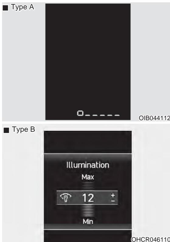
If the brightness reaches to the maximum or minimum level, an alarm will sound (if equipped).
