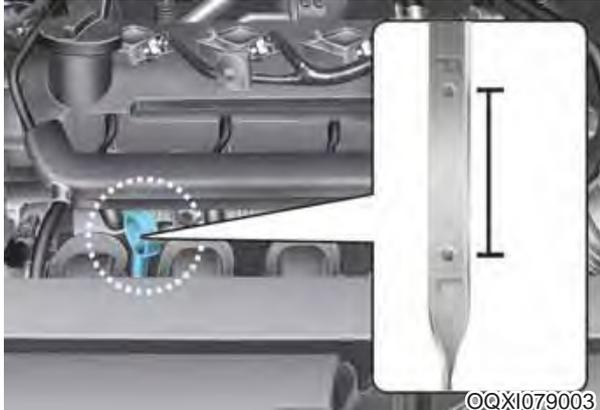
1. Be sure the vehicle is on level ground.
