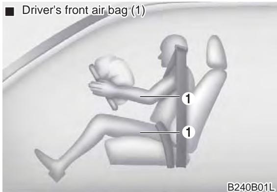
The air bag modules are located both in the center of the steering wheel and in the front passenger's panel above the glove box. When the SRSCM detects a sufficiently severe impact to the front of the vehicle, it will automatically deploy the front air bags.
