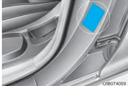
The vehicle certification label attached on the driver's (or front passenger's) side center pillar gives the vehicle identification number (VIN).
