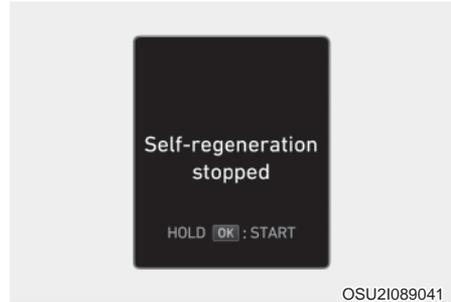
The self regeneration process stops if any of the self regeneration conditions is cancelled. If the self regeneration process is cancelled automatically, the system maintains "Self-regeneration stopped" message.
