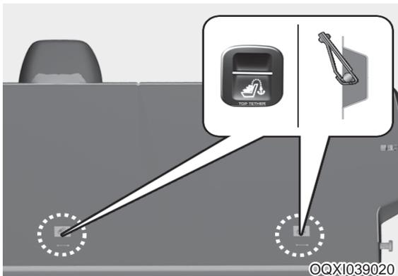
First secure the Child Restraint System with the ISOFIX anchorages or the seat belt. If the Child Restraint System manufacturer recommends the top-tether to be attached, attach and tighten the top-tether to the top-tether anchorage. Top-tether anchorages are located on the back of the rear seats.
