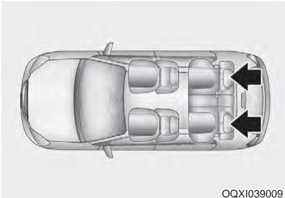
The rear seats are equipped with headrests in all the seating positions for the occupant's safety and comfort. The headrest not only provides comfort for passengers, but also helps to protect the head and neck in the event of a collision.
