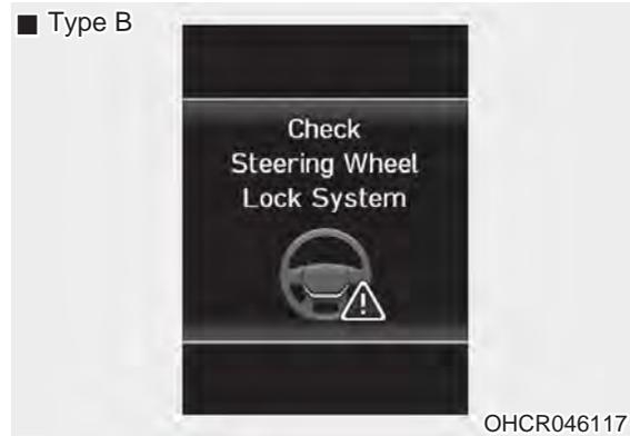
This warning message illuminates if the steering wheel does not lock normally when the Engine Start/Stop button is in the OFF position.
