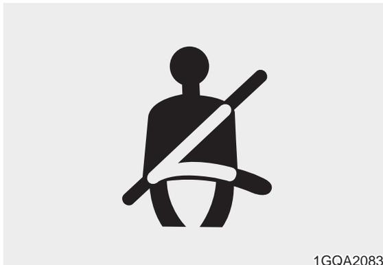
As a reminder to the driver or front passenger, the driver's or front passenger's seat belt warning lights will illuminate for approximately 6 seconds each time you turn the ignition switch ON regardless of belt fastening.
