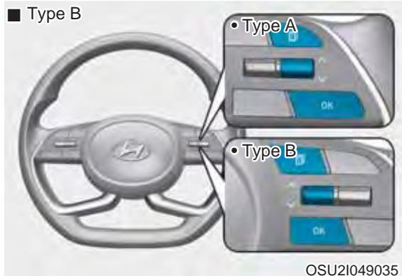
To change the trip mode, toggle the “D” switch on the steering wheel.
