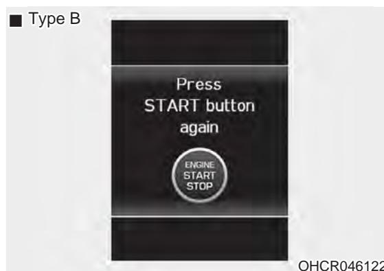
This warning message illuminates if you cannot operate the Engine Start/Stop button when there is a problem with the Engine Start/Stop button system.
