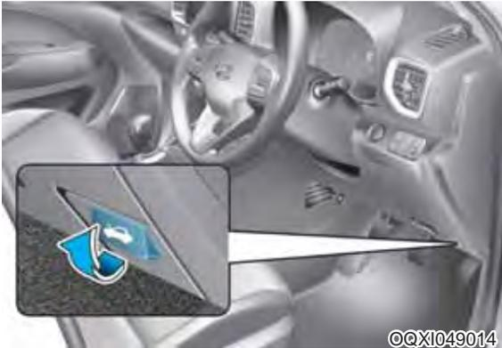
1. Make sure the shift lever is in P (Park, for Dual clutch transmission vehicle) or first gear or R (Reverse, for Manual transmission vehicle) and set the parking brake.
