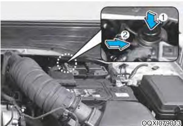
If you drive until you have no fuel left or if you replace the fuel filter, be sure to extract air from the fuel system as it makes it difficult to start the engine.
