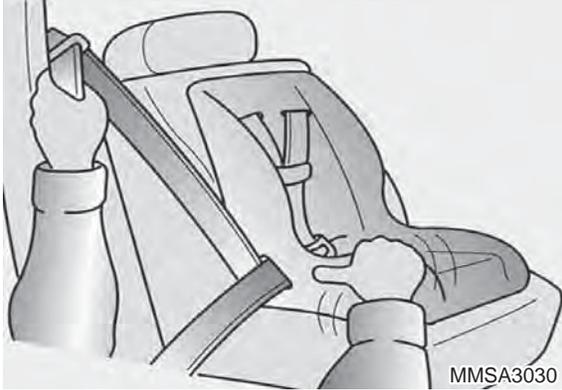
3. Buckle the seat belt and allow the seat belt to take up any slack. After installation of the child restraint system, try to move it in all directions to be sure the child restraint system is securely installed.
