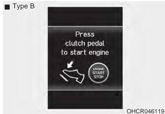
This warning message illuminates if the Engine Start/Stop button is in the ACC position twice by pressing the button repeatedly without depressing the clutch pedal.
