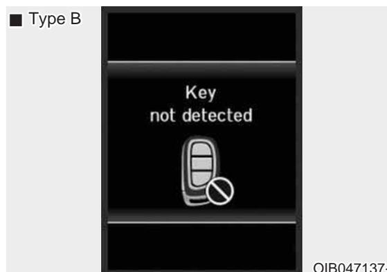
This warning message illuminates if the smart key is not detected when you press the Engine Start/Stop button.
