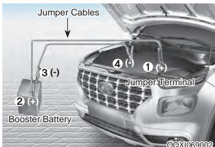
4. Connect the jumper cables in the exact sequence shown in the illustration. First connect one jumper cable to the red, positive (+) jumper terminal of your vehicle (1).
