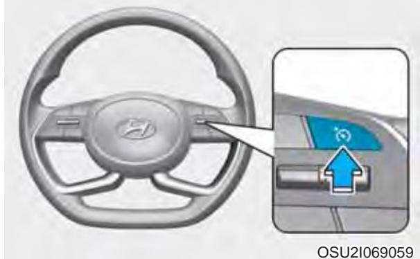
1. Press the CRUISE button on the steering wheel to turn the system on. The cruise indicator will illuminate.
