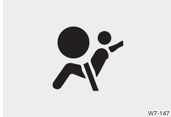
The purpose of the air bag warning light in your instrument panel is to alert you of a potential problem with your air bag - Supplemental Restraint System (SRS).
