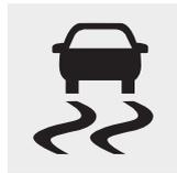
When the ESC is in operation, the ESC indicator light blinks:
