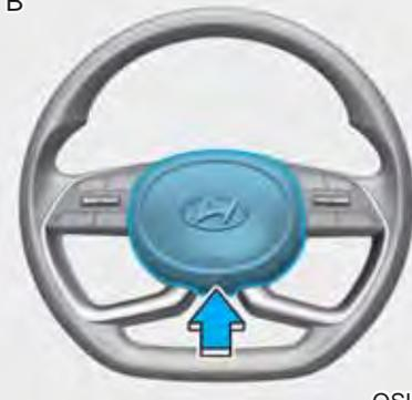
To sound the horn, press the area indicated by the horn symbol on your steering wheel (see illustration). The horn will operate only when this area is pressed.
