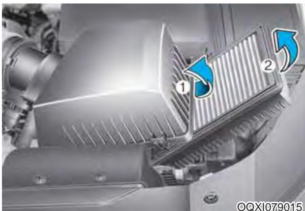
2. Remove the used filter and wipe the inside of the air cleaner housing carefully not to remain dusts in the cover housing.
