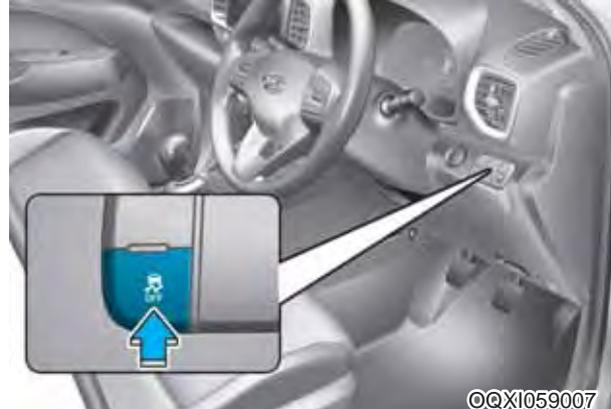
The Electronic Stability Control (ESC) system helps to stabilize the vehicle during cornering maneuvers.
