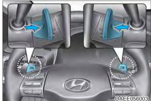
The paddle shifter is available when the shift button is in the D (Drive) position.
