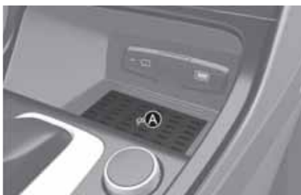
[A] Vehicle authentication pad (Wireless charging pad)
