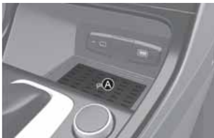
[A] Vehicle authentication pad (Wireless charging pad)
