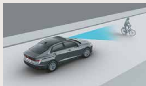
Forward Collision - Avoidance Assist - Cycle (FCA-Cyl)
