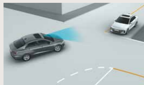
Forward Collision - Avoidance Assist - Junction Turning (FCA-JT)
