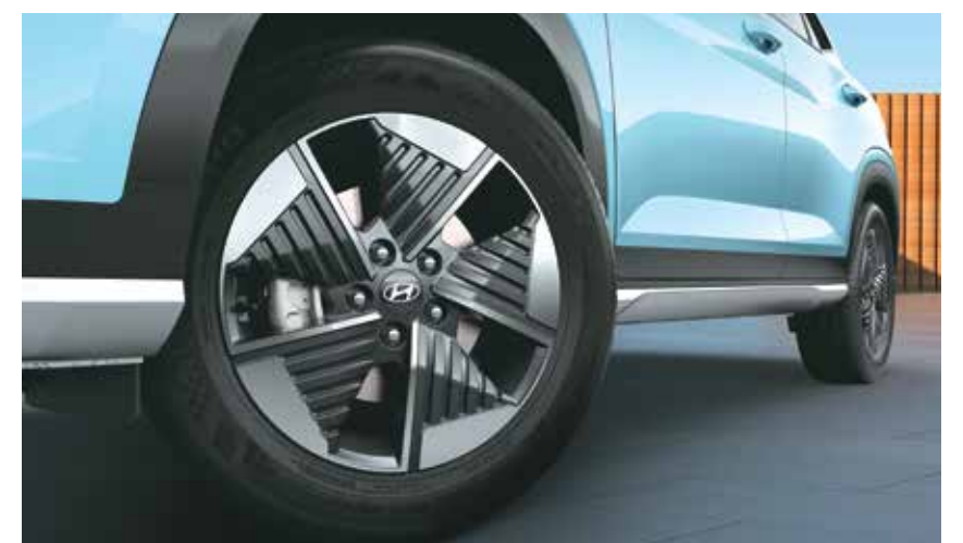
R17 (D=436.6 mm) Aero alloy wheels with Low Rolling Resistance (LRR) tyres
