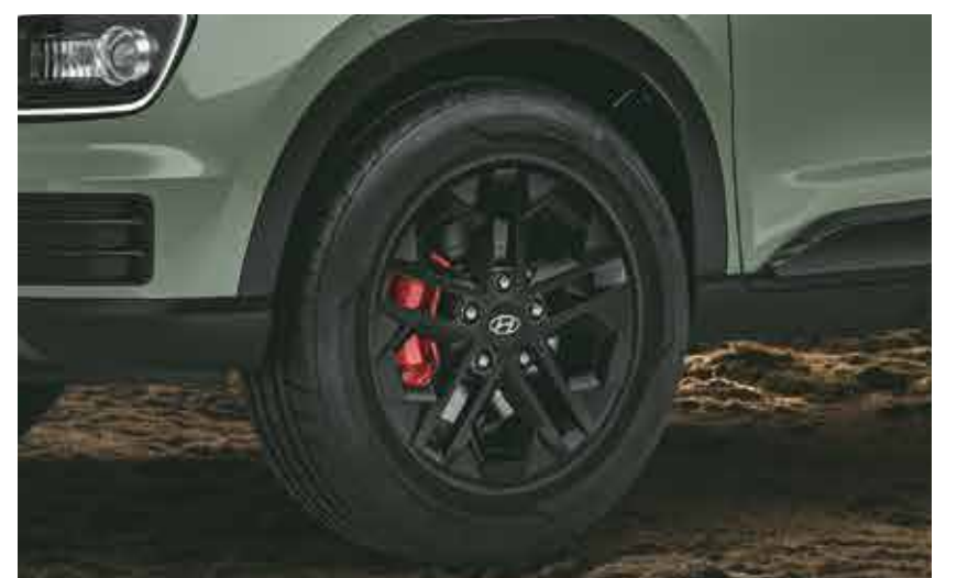
Black painted alloy wheel with red front brake caliper
