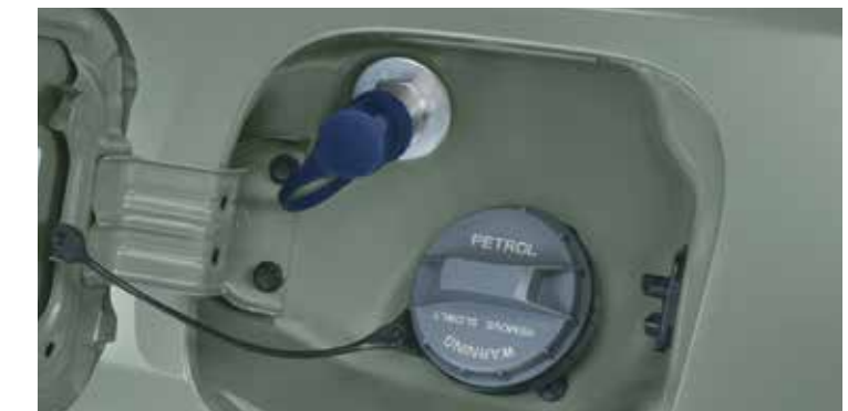
Convenient CNG filling with fast refueling nozzle (near petrol filling area)
