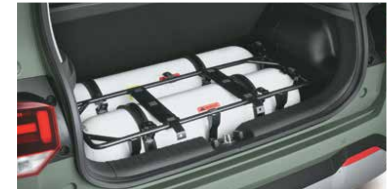
Company fitted dual cylinder CNG
