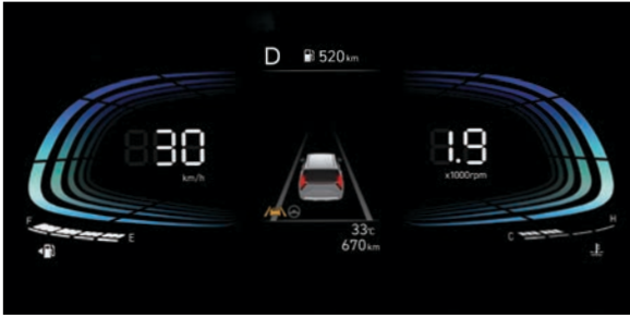
Full Digital Supervision Cluster with 4.2" TFT LCD
