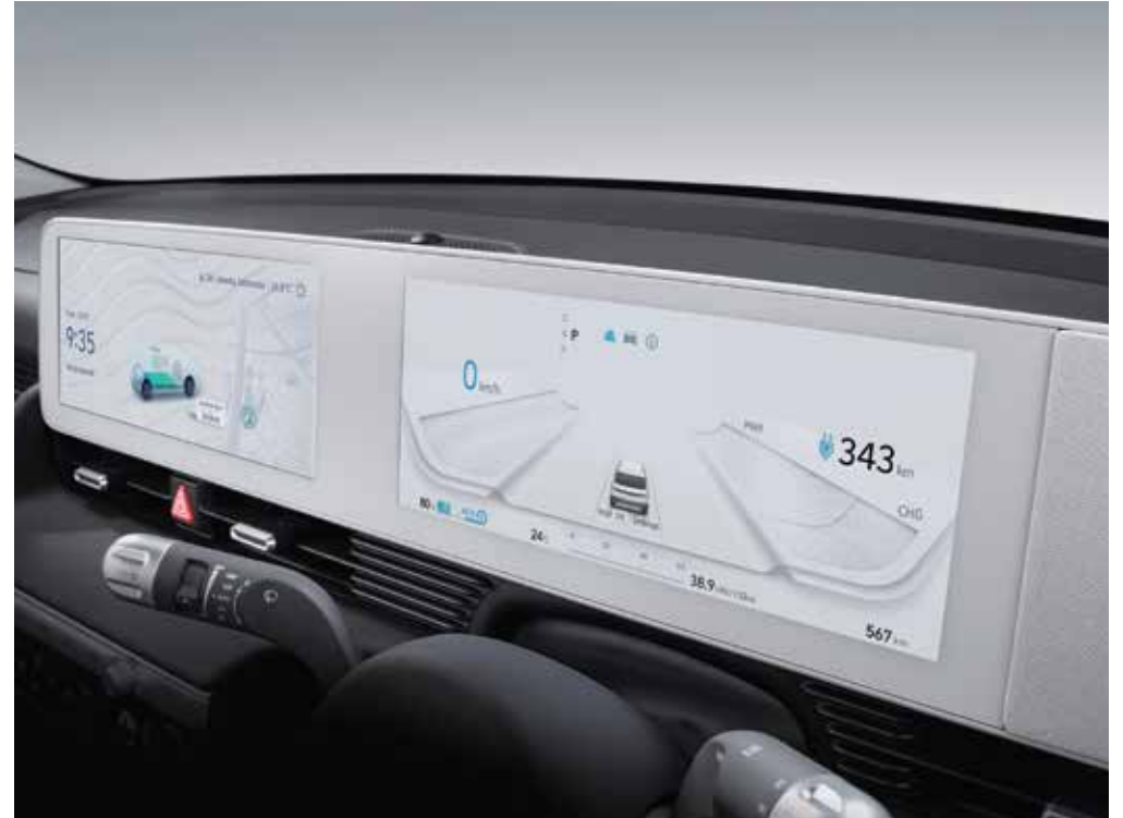
12.3" TFT LCD Cluster with integrated A/V System
