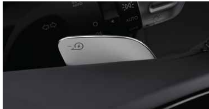
Paddle Shifter for Regenerative Braking
