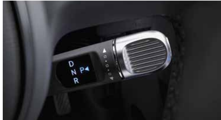
Column Type Shift-By-Wire
