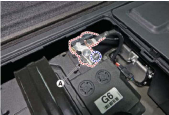
4-2. Turn the ignition switch OFF and disconnect the auxiliary 12V battery negative (-) terminal (A).
