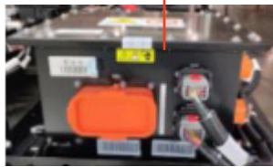
High-voltage Junction Box
