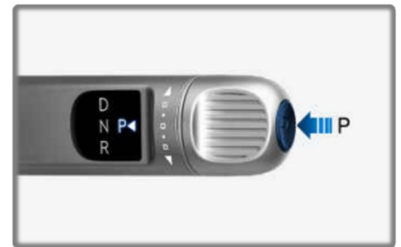
Put the vehicle in P (Park) position by pressing the 'P' button on the rotary shifter
